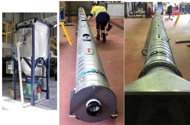
Figure 5. Pilot filters, Left: 1 m rapid pulse unit, Right: 9 m gas flow analyser.
