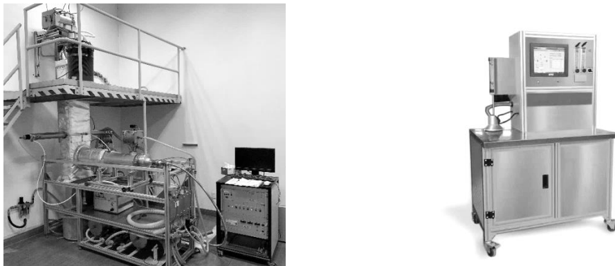
Figure 6. Filter media efficiency testers, Left: rapid pulse unit, Right: micro fine dust unit.
